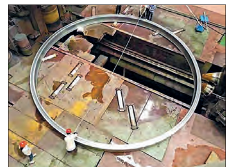
Fig. 5: The 10-m aluminium alloy ring is to be used in heavy-lift rockets
